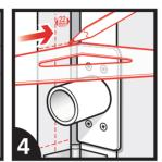
Mark the top and bottom edges level and square across to the door frame. Mark a centre line 22mm from the knuckle side of the frame.
