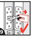
Remove the retaining plate. Ensure that it is kept in a safe place in case it is necessary to remove the closer from the door at any time.
