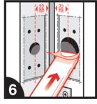
Cut out the area required to house the fixing plates on both the door leaf and the door frame.
