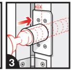
Drill the hole for the closer body using the auger bit. Do not drill to excess, the door control should be a snug fit.
