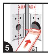
Cut out the area required to house the fixing plates on both the door leaf and the door frame.
