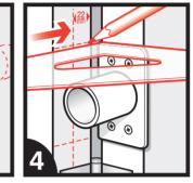
Mark the top and bottom edges level and square across to the door frame. Mark a centre line 22mm from the knuckle side of the frame.
