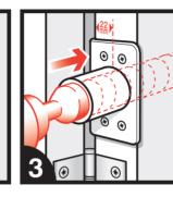
Drill the hole for the closer body using a Lewis auger bit.
