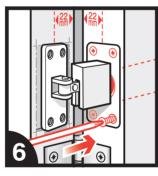
Insert the body of the closer into the door leaf, with the retaining block facing you, and screw fix.
