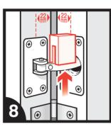
Remove the retaining block. Ensure that it is kept in a safe place in case it is necessary to remove the closer from the door at any time. Depending on the handing of the door, the retaining block will push up or down.
